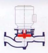
Applicable for pumping liquids contaminated with solids not greater than 15 mm in size. and the maximum medium density is 1300 kg/m<sup>3</sup>. Used in food processing and sugar industry, chemical industry, for sludge, slurries and washings pumping, also as pump for lime milk and synthetic resin dosage.
