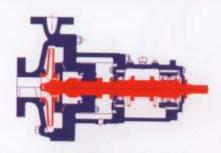
Applicable for pumping petrochemical products, chemicals and hot water, of temperature up to 400°C. Mainly used in oil refineries, chemical industry and in explosion hazardous areas.
