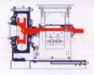
Applicable for hydraulic transport of sand, gravel, non-ferrous metals ores, flotation tailings, ash, coal, lime milk; for pumping highly abrasive mixtures of water and solids not greater than 15 mm in size. The maximum slurry density is 1600 kg/m². Used for copper ore pumping in flotation process, in mining industry, sugar industry and in other applications, where high pump abrasion and erosion resistance is required.
