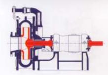
Applicable for hydraulic transport of sand, gravel, stones, coal, slag, ores, ash, clay, lime milk, flotation tailings etc., for pumping highly abrasive mixtures of water and solids not greater than 52 mm in size. The maximum slurry density is 1700 kg/m³. Used in coal mines, in minerals and ore mines, power plants, steel works, cement mills, lime mills, sugar plants, solid waste disposal systems, etc.
