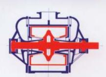
Applicable in food processing industry, paper industry, chemical industry, in filtration and distillation processes and for gas compression. Used also in sugar plants, and to provide the vacuum in evaporation process.
