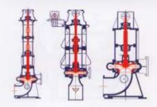
Applicable for pumping water contaminated with solids, industrial and municipal waste water. The maximum solid size is 100 mm and the maximum medium density is 1100 kg/m3. Mainly used as pumps for industrial and municipal waste water handling systems.
