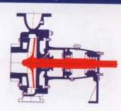
Applicable for pumping technological liquids slightly contaminated with solids (not containing fibers), for mechanically treated waste water and for suspensions of dry mass concentration not exceeding 3%. Able to handle gas evaluating liquids and viscous liquids of temperature up to 150°C. Used in food processing industry, for pumping lime milk, sugar juices and mechanically treated waste water.
